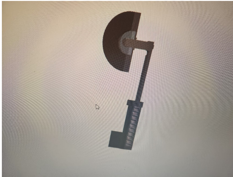
Figure 11: Section Cut of Original Piston Tensioner Design
